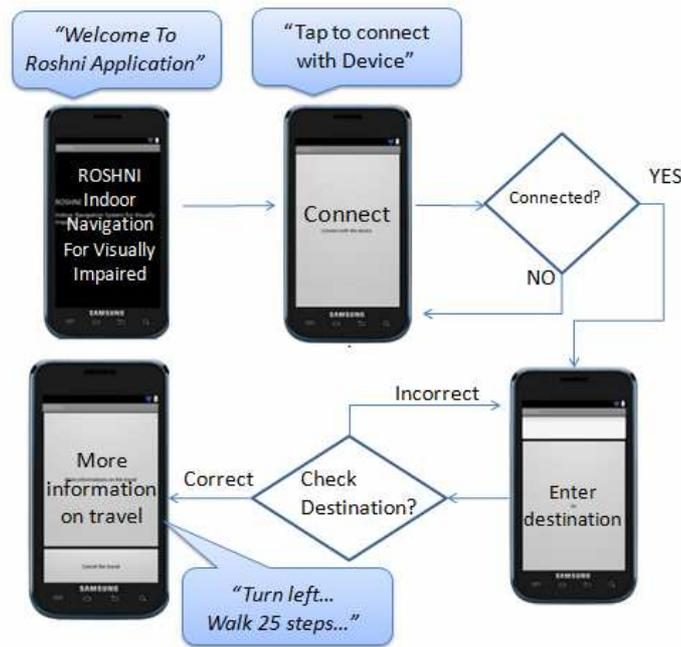
**Figure 4: Flow diagram illustrating the audio-based user interface.**
