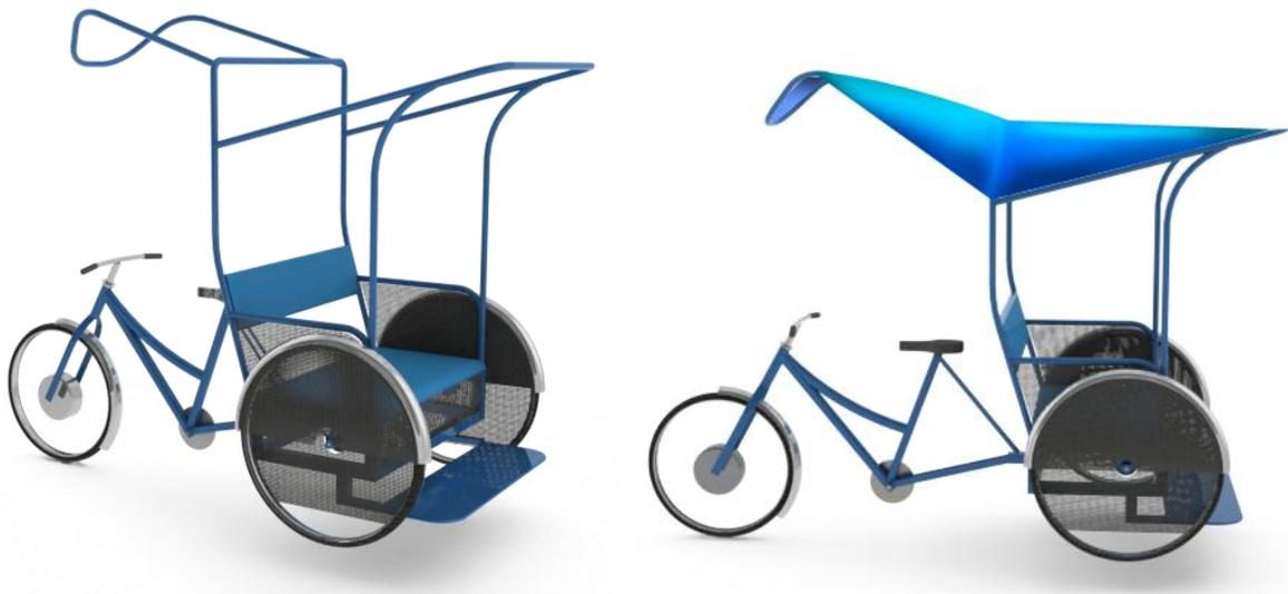
*conceptual CAD model showing protection guard near wheels*
